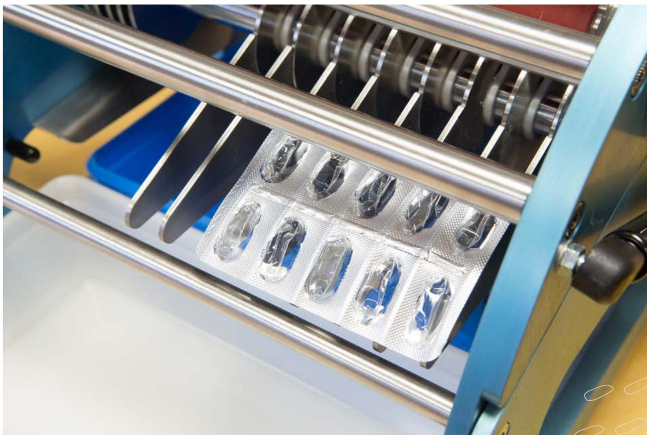
Stripfoil Mini is a compact, manually operated deblistering device. It offers a practical and cost-efficient way of processing small quantities of medication.
