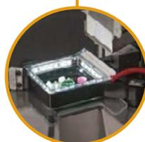
Verification of correct placement by optical sensors.
